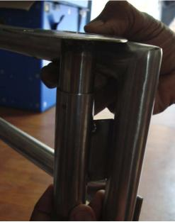
B) Inner holding tube needs to be screwed on to the fiber cover after you drill a hole in the SS frame and thread it for one of the sides
