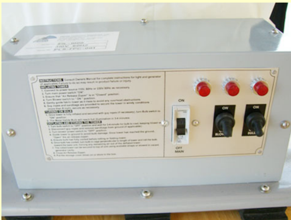
Figure 4: The control switch device, comprising: a power switch (left), inflatable UP switch (middle) and lighting start switch (on the right).
